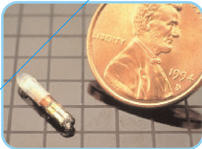
6. Applied Digital Solutions' VeriChip, which is smaller than a penny, can be embedded under a patient's skin. Using RFID technology, this biometric chip gives medical personnel instant access to a patient's medical records.
