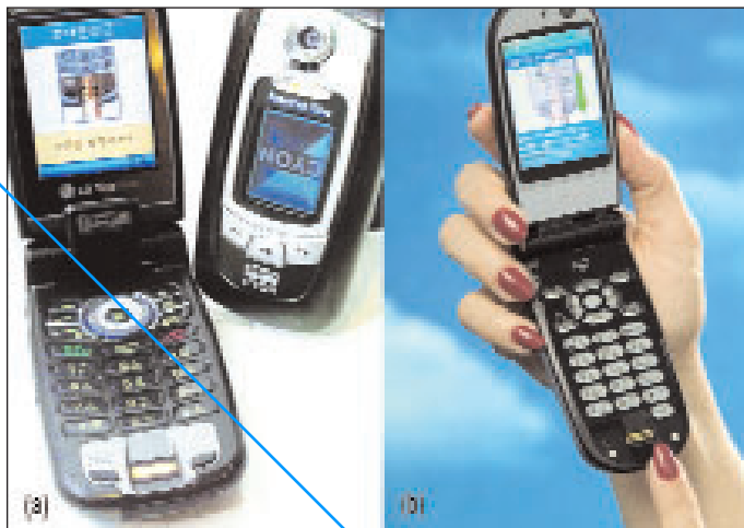
5. Biometrics sensors are finding greater use in consumer electronics items like cell phones. LG Electronics' 3550 and 3800 cell phones (a) and NTT Docomo's 900iC cell phones (b) are just a couple of examples. These phones use AuthenTec's EntréPad 1530 optical sensor.
